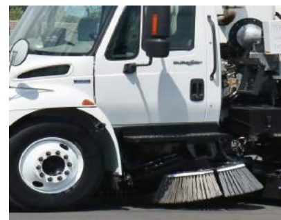
Gutter brooms sweep debris to the middle.
