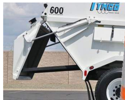
Pick-up brooms load debris into the hopper.
