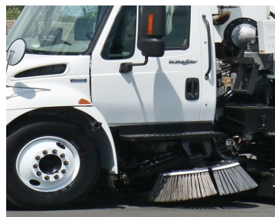
Gutter brooms sweep debris to the middle.
